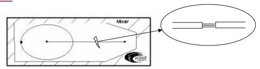
The design for the mixer provides a junction for two solutions to combine along a path length of 12mm. The mixed solutions are filtered further down the micro channel through a restrictor and may be collected.
