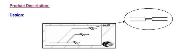
The Microfluidic Auto Dilution chip serves as an on-chip auto dilution and filtration system. A solution injected into the input port is automatically split into three channels and is filtered upon passing through frits in each micro channel.
